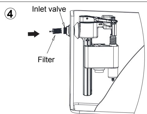
Reinstall the filter and the water supply pipe.
