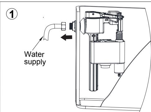
Turn off the water supply, screw off the water supply pipe.
