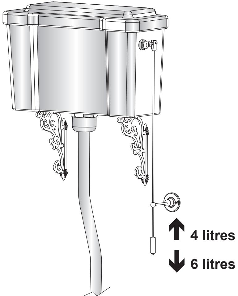
**Please note that it is imperative that there are no loops or kinks in the yellow tube when installed and that the lever is not operated with excessive force as this will damage the cable inside the tube that lifts and lowers the flush valve causing the flush to fail beyond repair**
