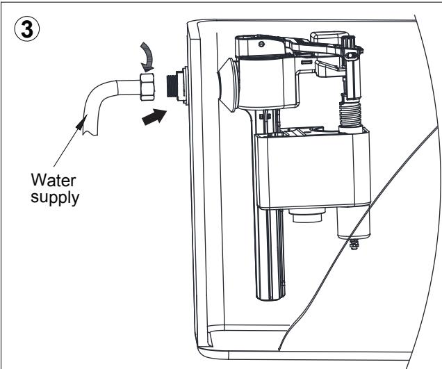
Tighten the nut, connect the water supply to the cistern.
