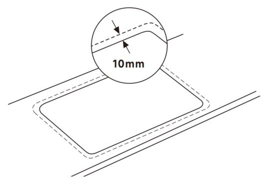
2. Cutting the Opening Use a jigsaw to cut the opening along the marked lines
