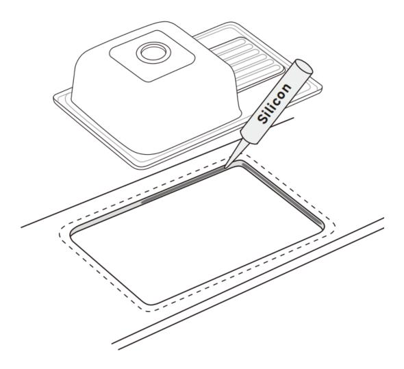
Use kitchen-safe silicone, such as glazing silicone The silicone serves two purposes: Sealing the edges against moisture Holding the sink in place
