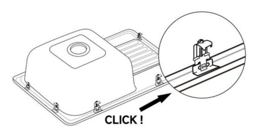
If there are no clips, the sink will be secured solely with silicone Press the sink firmly to ensure proper adhesion
