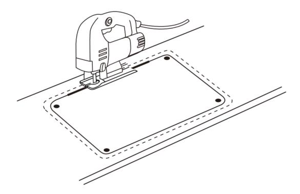
Be precise and careful to ensure the cutout matches the sink's dimensions Always wear protective goggles and gloves when cutting
