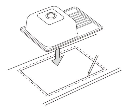
Trace its outline carefully Inside the drawn shape, mark a second outline 8–10 mm smaller to create a proper support edge
