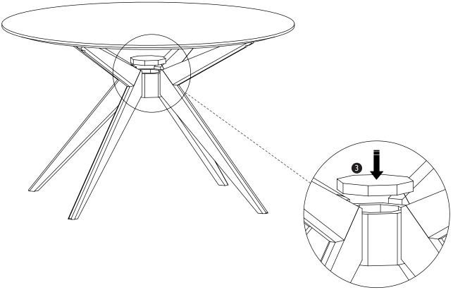
Please note that the octagon shape between the wooden cover (part 3) and the wooden column (part 4) should align.
