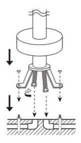
3. Connect the flexible hoses tightly to the main faucet body. Then connect both body elements together.
