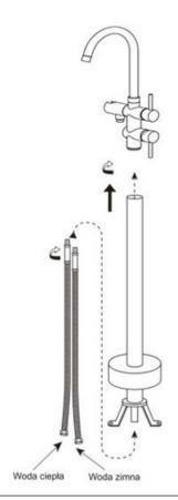
5. Install the shower hose and hand shower. Carefully check the installation and the tightness of all faucet components.
