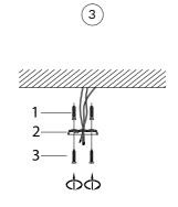
Drill holes apply plastic anchors
