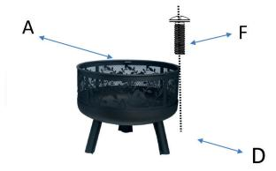
Connect the legs(D) and the fire bowl (A) with 9pcs  $$\tt screws(F)$$
