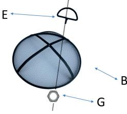
Connect the mesh cover handle (E) and the mesh cover (B) with nut (G)  $\,$
