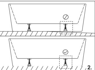
• Check that the position of the tub is horizontal. Adjust the legs of the bathtub to compensate for level differences.
