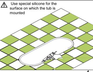
• Apply a thick layer of silicone inside the marking.
